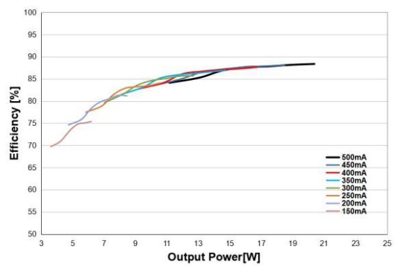
IT FIT 20 500 CS Independent Typical Efficiency vs Load
