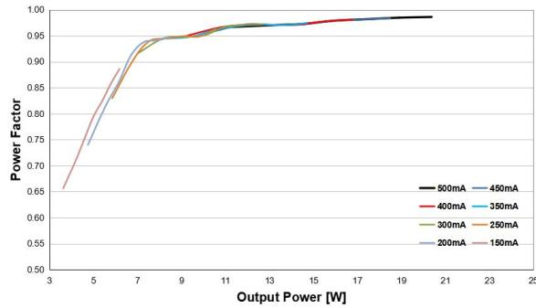
IT FIT 20 500 CS Independent Typical Power Factor vs Load
